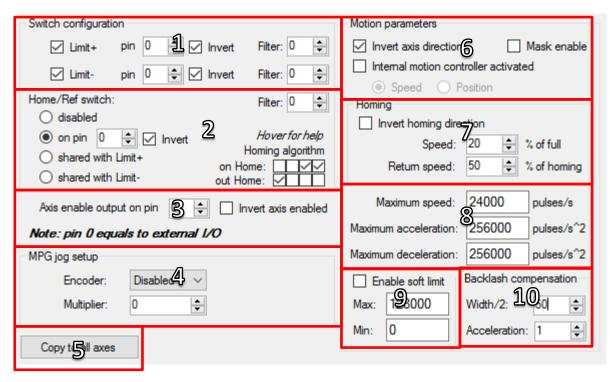
Figure 4: Axis configuration panel
