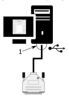
**Step 1**: Locate a free USB 2.0 port on your computer (1) and connect PoKeys57CNCdb25 board (2) to it
