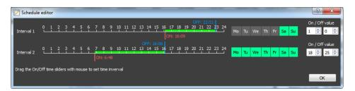
In order to allow remote schedule modification, 'Expose rules values' option is available. Additional rules outputs appear on the block, which can be connected to Shared data slots. The rule is bit-wise encoded in a 32-bit value as described in the list below:
